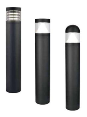
Palo 25 is a modern architectural, directional optically controlled bollard which is constructed from cast aluminium with a IP65 rating. Robust design with optical distribution and suitable heads such as Dome, Flat and Louvred. Available with a flange or root mounted kit.
